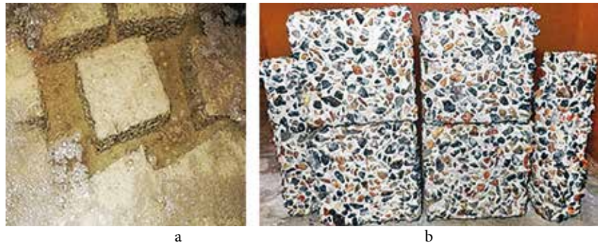
Figure 3.5. Specimens after being soaked in the sulfuric acid solution (a): Soaking in the acid solution; (b): After removing the corroded layer
