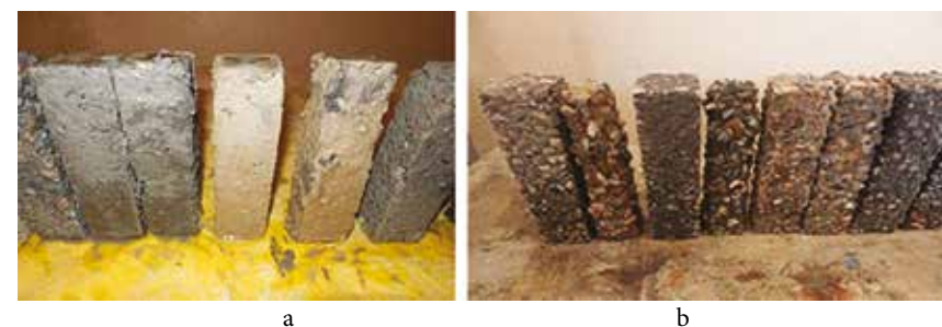
Figure 3.7. Specimens after being soaked in a 5 % solution of sulfuric acid: (a) before cleaning; (b) after cleaning corrosion products
