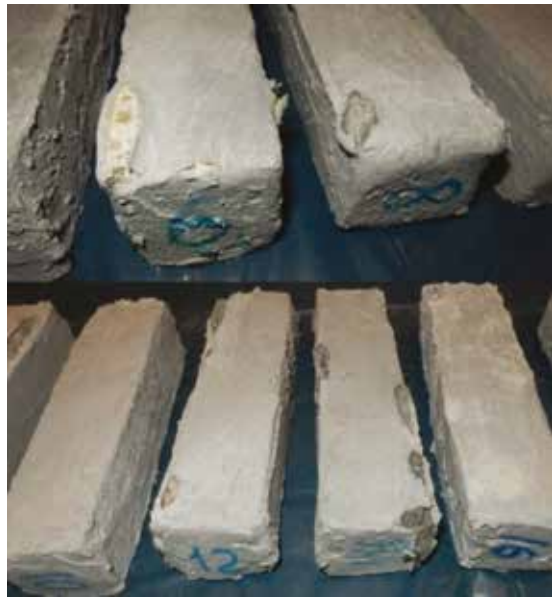
Figure 3.10. Specimens with epoxy coating after 120 days of exposure to acid
