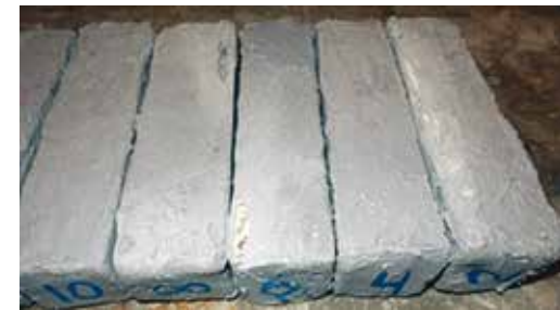
Figure 3.8. Specimens with epoxy coating after 60 days of exposure to acid
