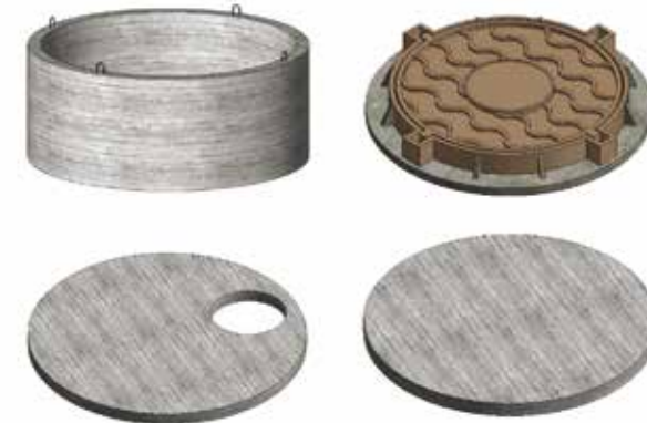
Figure 6.47. Families designed to assemble inspection manholes
