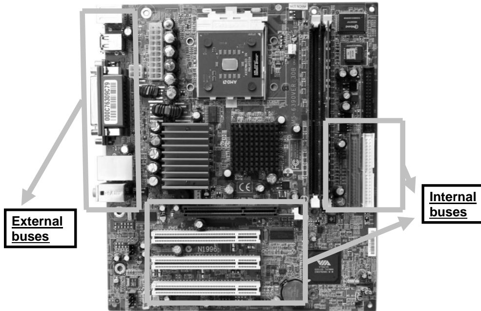
Fig. 2.6. Position of computer buses on the motherboard
