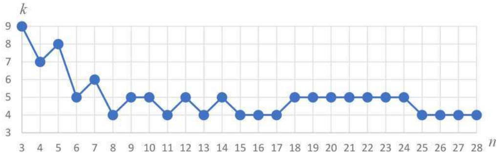
Fig. 12. The number of iterations of the circle-based partitioning algorithm for the curve in Fig. 4 as n varies from 3 to 28, with allowable chord length deviation \varepsilon = 0.0001 and n_1 = \lfloor n/2 \rfloor
