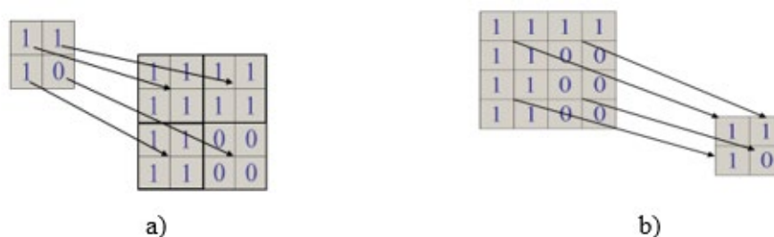
Figure 4 - Operations of increasing (a) and decreasing (b) the size of a binary image when scaling
